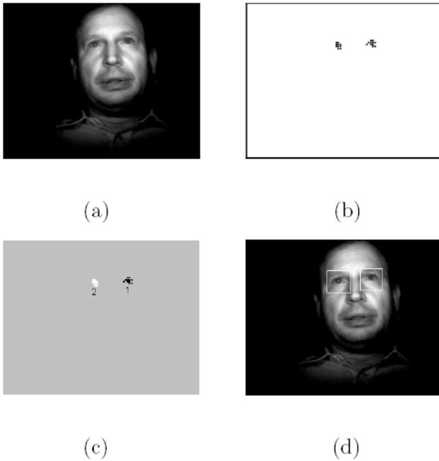
Figure 8: Eye Localization Algorithm (a) original image, (b) network response, (c) clustered network response, (d) eye windows
