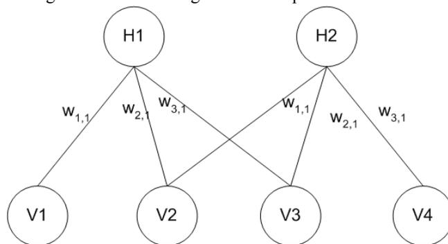
Figure 3: Each unit in layer H is connected by the same three weights to three units in the previous layer (V)
