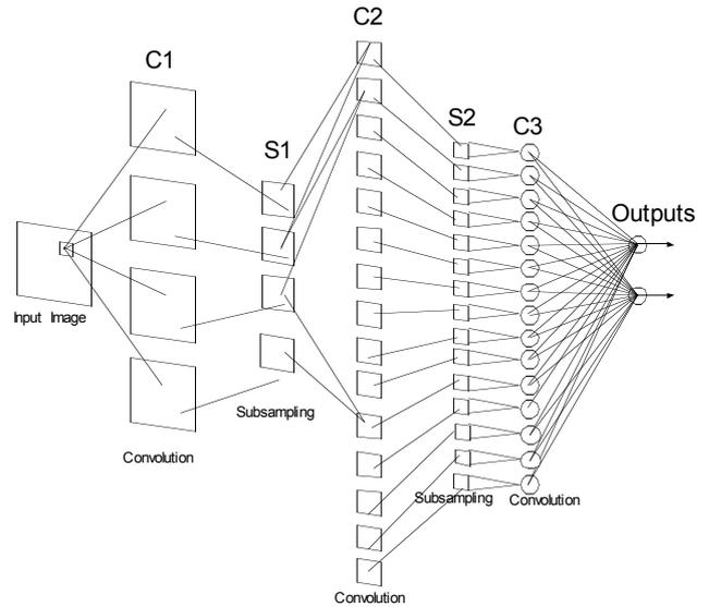
Figure 4: CNN Architecture for Eye Detection
