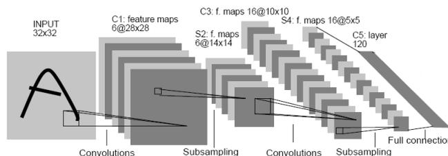
Figure 2: A Typical Convolutional Neural Network [23]
