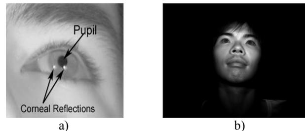
Figure 1: Eye Tracker's Images a) small field of view, b) larger field of view
