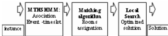
Fig. 1. An instance of the problem is received like input, this it happens through an association process event-timeslot, assigns events to a timeslot, later a matching algorithm [8] is used for makes the assignation from rooms to each one of events associated to timeslot. In this point a solution is complete, but is low quality. Then a local search algorithm [12] is applied that improves the quality of the solution and gives like final result one optimal solution to the UCTP.
