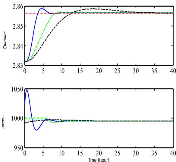
Fig. 5. Closed-loop system response to a desired steady state output flow rate of 2.8566 m<sup>3</sup>/s due to the effect of non-constrained MPC (solid), constrained MPC dash-dotted and PID controller (dashed)
