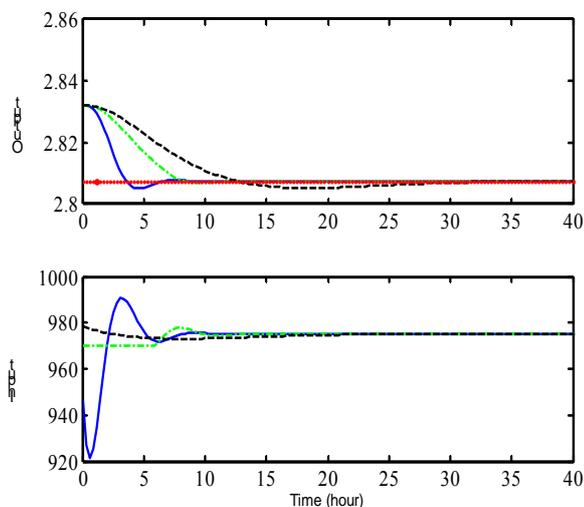
Fig.6. Closed-loop system response to a desired steady state output flow rate of 2.8074 m<sup>3</sup>/s due to the effect of non-constrained MPC (solid), constrained MPC dash-dotted and PID controller (dashed)
