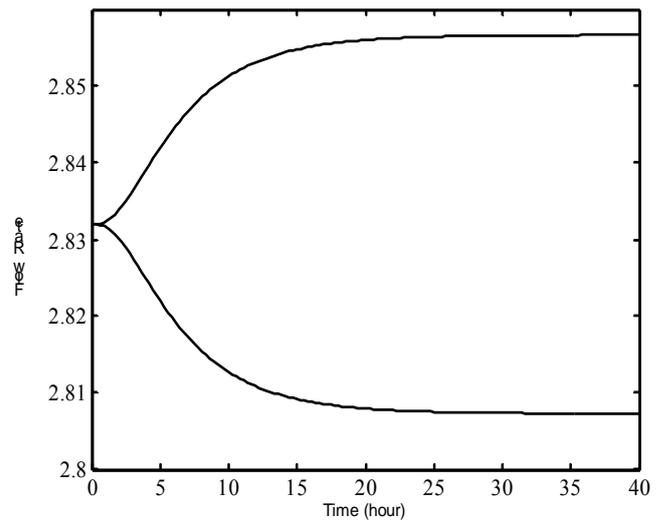
Fig.3. Output flow rate  $Q_o(t) \text{ m}^3/\text{s}$  for  $N = 985 \pm 10\%$  rpm square wave speed variation
