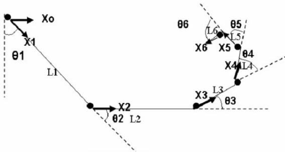
Fig. 1 Frames on each joint.
