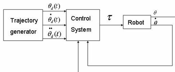
Fig. 7 High-level Block Diagram of a Robot Control System
