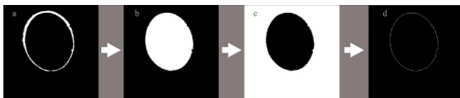
Fig. 8 Test tank edge detection procedure. (a) Test tank detected by the sensor. (b) Filling result by region grow. (c) Inner boundaries of the test tank after logical operations. (d) Edge detected by Canny for mapping only.
