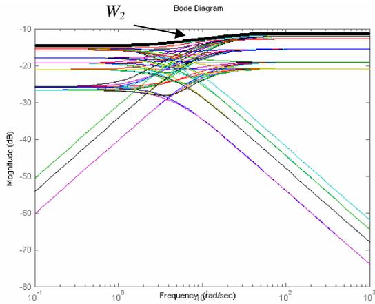
**Fig.1** The design of uncertainty weight of DC motor speed control plant.
