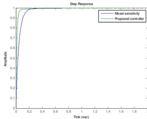
**Fig. 3** Step responses of the proposed optimal PID controller and a conventional robust controller at a nominal plant.
