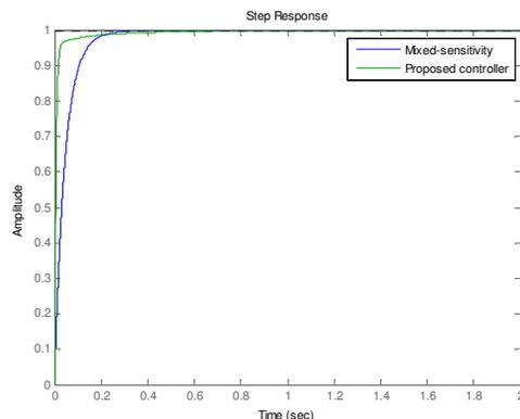
**Fig.4** Step responses of the proposed optimal PID controller and a conventional robust controller at a perturbed plant.
