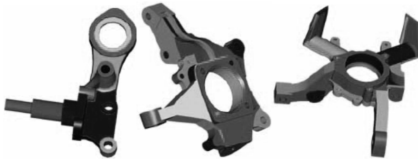
FIGURE 1 FROM LEFT TO RIGHT THE DIGITIZED MODELS OF THE FORGED STEEL, CAST ALUMINUM AND CAST IRON STEERING KNUCKLES.
