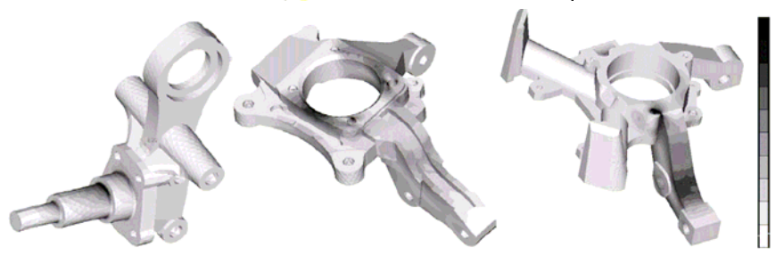
FIGURE 2 EQUIVALENT VON MISSES STRESS CONTOURS AND CRITICAL LOCATIONS FOR A TYPICAL LOAD VALUE
