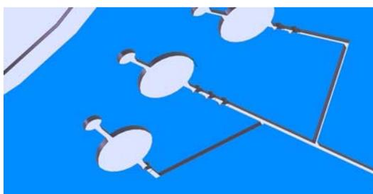
Fig.1: Sketch of the proposed well-type valves. The first zone is loading hole and reservoir is the next, then it is the well-type valves.
