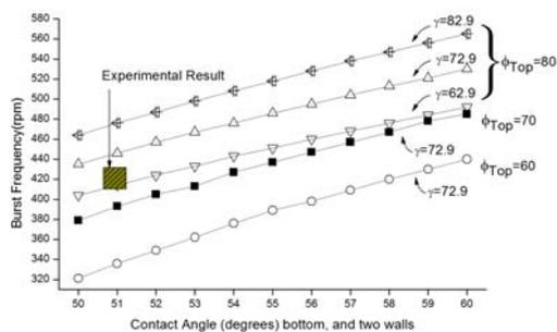
Fig. 5: The comparison of theoretical and experimental burst frequency. Contact angles inside channel surfaces, such as side and bottom walls, covered scotch tape, are measured by separated equipment.
