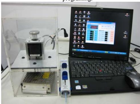
Fig.3: Schematic of Experimental Setup for Burst Frequency Measurements. The computer can control the motor RPM in different connected priffle
