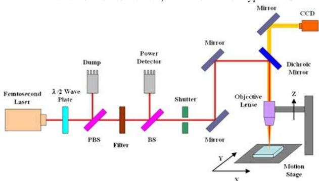
Fig.2: The experimntal setup of femtosecond laser. The CD-ELISA is located on the motion stage. Three axes can be moved using NC programming.
