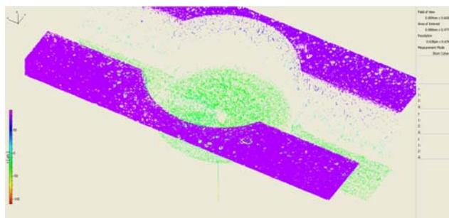
Fig. 4: The 3D well-type valve is fabricated by the femtosecond laser. The hole is about 50um and it is used in a 25um micro channel.
