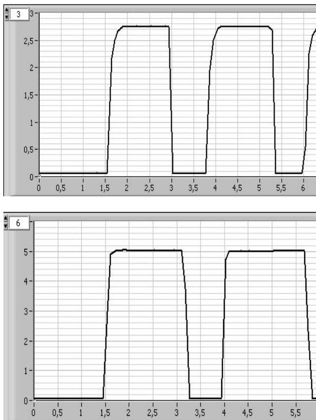
Fig. 8 Evolution of pressure in the tested pneumatic muscles
