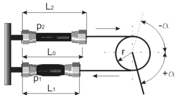
Fig.3. Kinematics of the rotation module
