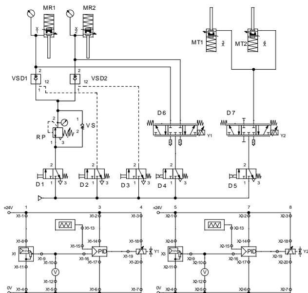
Fig. 6. Control diagram of the pneumatic muscles
