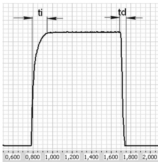
Fig. 9. Determining inflation/deflation times
