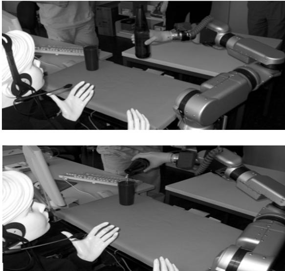
Fig. 1. Pouring drink into a glass by means of vocal control
