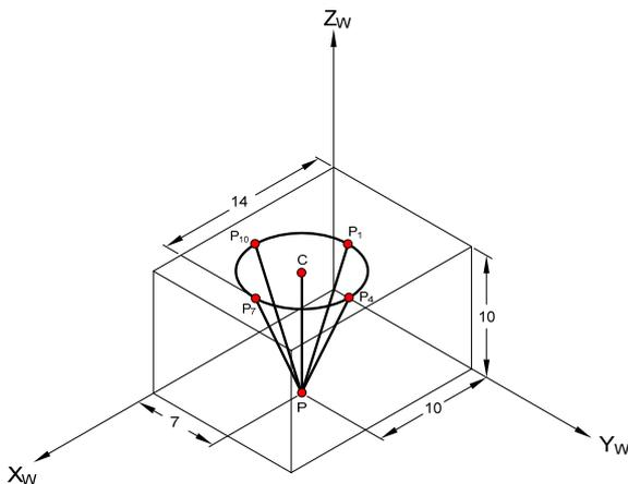
(a) dimensions of a work-piece for making a conical part
