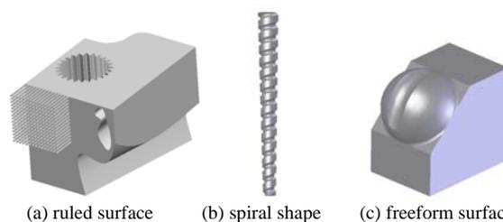
Figure 6 The feasible machining geometric features by the innovative mechanism
