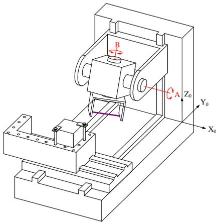
Figure 7 A new configuration of 5-axis WEDM
