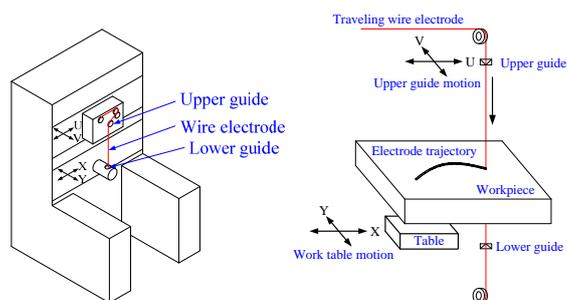
Figure 1 5-axis WEDM structure [2]
