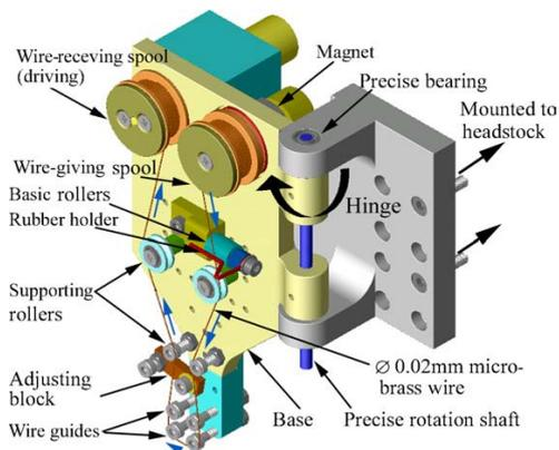
Figure 3 Wire electrode guide mechanism [4]
