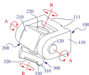
Figure 5 Innovative mechanism module for wire electrode [6]
