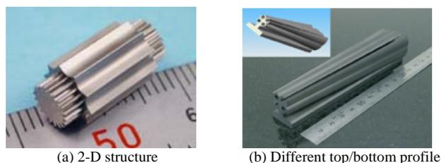
Figure 2 Parts made by existing 5-axis WEDM [3]
