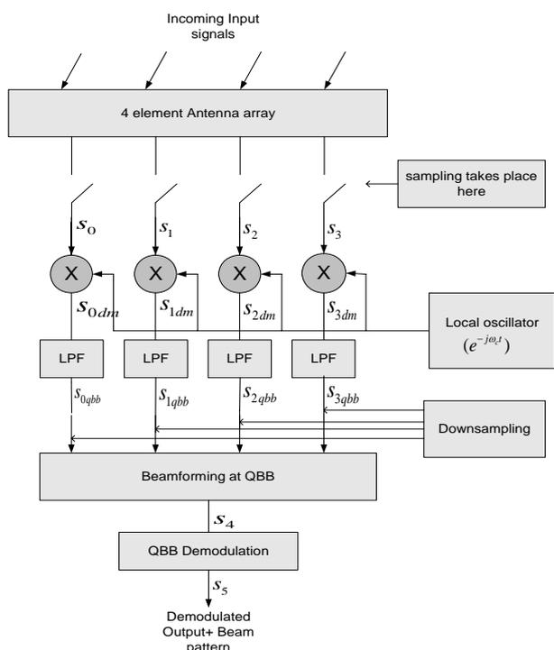
Figure 2: Beamforming at Quadrature baseband
