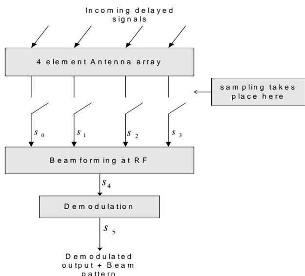
Figure 1: Beamforming at radio frequency
