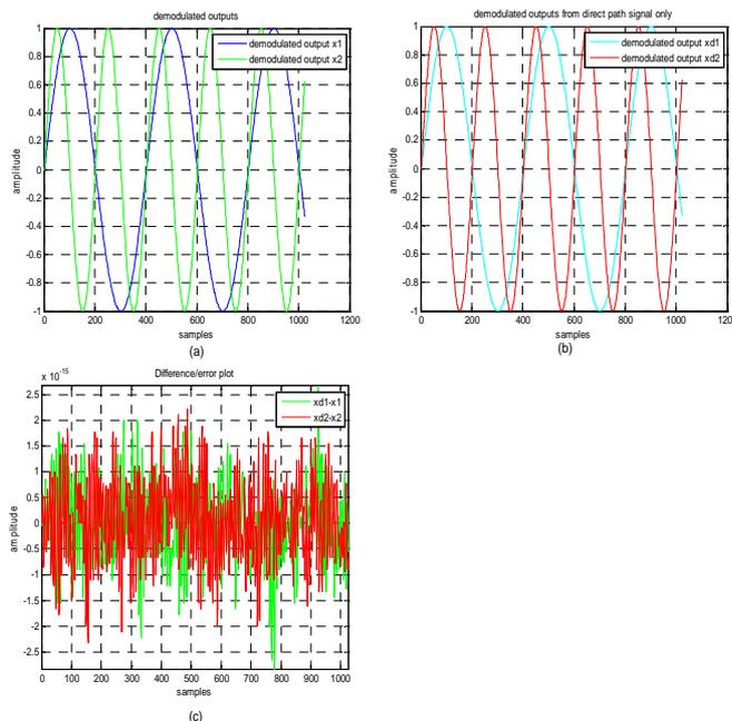
Figure 6: (a) Compensated signal demodulated output: the compensated modulated output was demodulated and gives this signal output. (b) Direct path signal demodulated output: this signal output facilitates for measuring of the accuracy of the compensation process by plotting its difference from the compensated demodulated out put. (c) Difference/error plot: has a very small value of about  $2.5e-14$  shows a very insignificant difference which entails a successful compensation was done.
