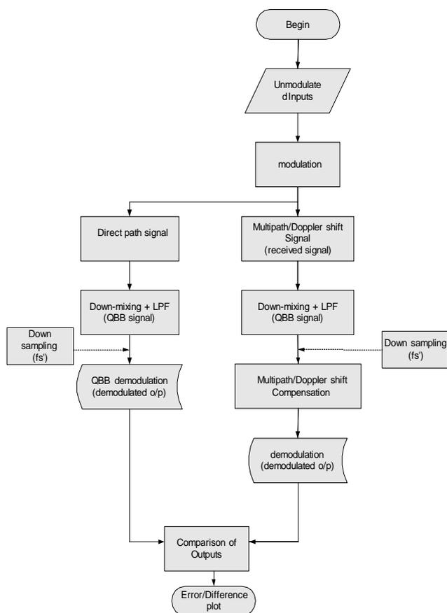
Figure 5: Multipath/Doppler shift compensation at QBB
