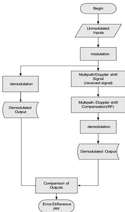
Figure 4: Multipath/Doppler shift compensation at RF
