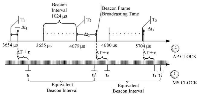
Fig. 5 Synchronization Between APs and MSs
