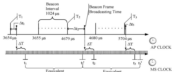
Fig. 4 Beacon Frame Transferring Time Measurement Resolution Improvement
