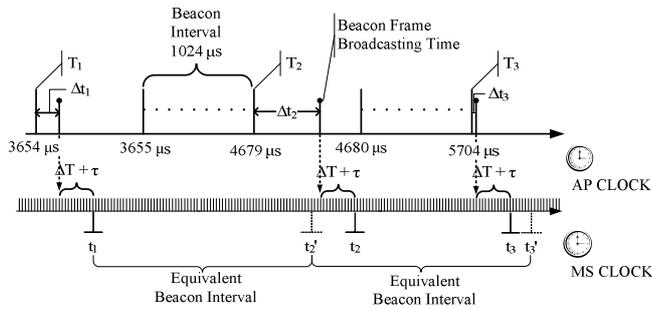
Fig. 5 Synchronization Between APs and MSs
