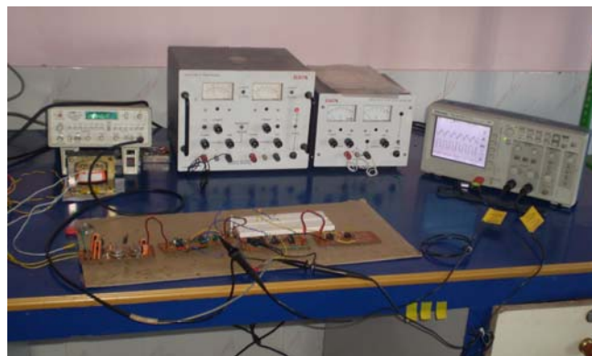
Figure 3: Basic arrangement of Phase Locked Loop
