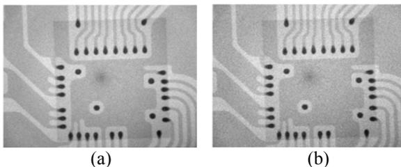
**Fig. 5:** (a) Original image from X-Ray camera, (b) Image with additive Gaussian white noise variance  $\sigma = 0.015$
