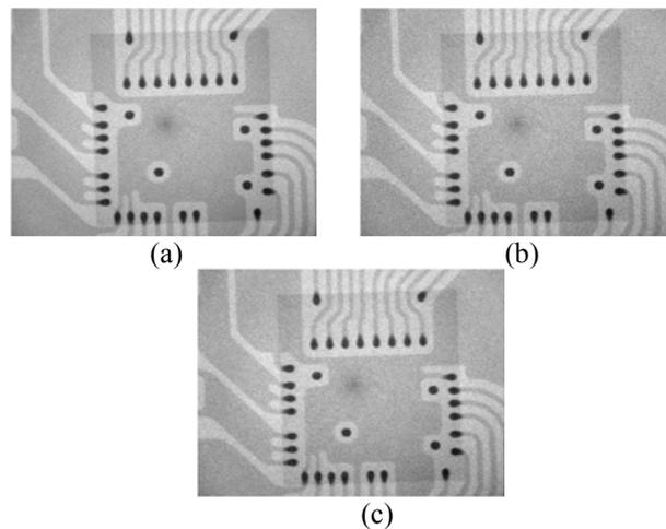
**Fig. 7** (a) Original image from X-Ray camera, (b) Image with additive Gaussian white noise  $\sigma = 0.015$ , (c) 2<sup>nd</sup> iteration of applying Fuzzy filter with  $\alpha = 2.13$ .
