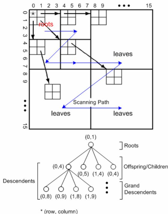
Figure 2. The SOT structure adopted by SPIHT.
