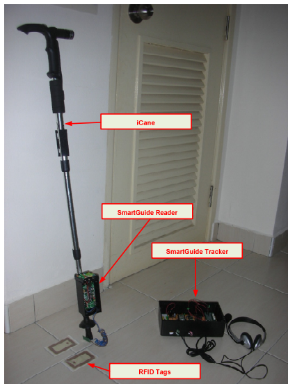
Figure 3. Block diagram of SmartGuide RFID component attached to cane.
