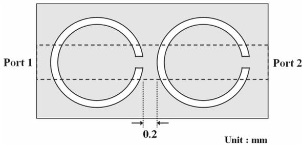
Fig. 3. Top view of the two slotted ground structures underneath the microstrip line. (Dimensions of the two SGSs are the same with Fig. 1(a))
