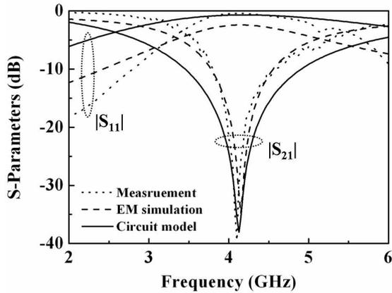
Fig. 2. Frequency responses of circuit simulation, EM simulation and measurement for the single slotted ground structure. ( $r_{ext} = 5.2$  mm,  $g = 2$  mm and  $w = 0.6$  mm in Fig. 1(a))
