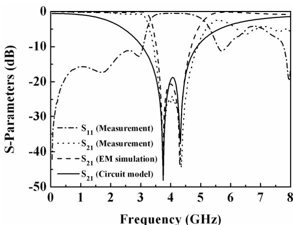
Fig. 6. Frequency responses of circuit simulation, EM simulation and measurement for the two slotted ground structures.
