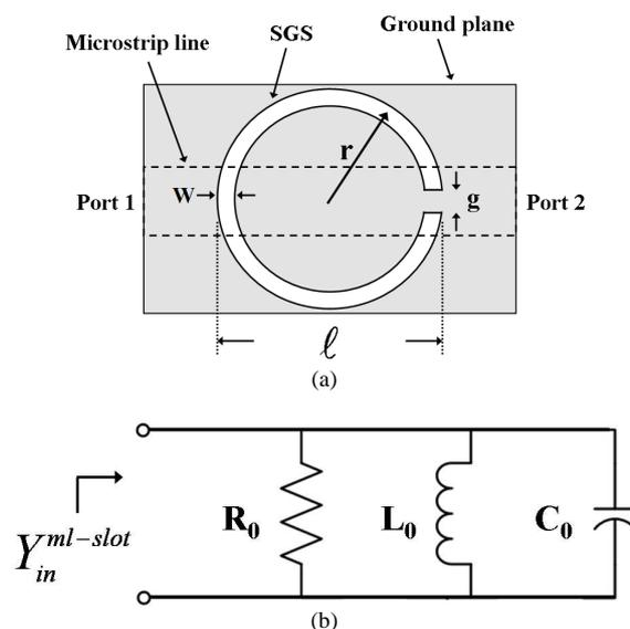
Fig. 1. (a) Top view and (b) the equivalent circuit model of the single slotted ground structure. (The gray is the metallic conductor and the white is the etched ground plane)
