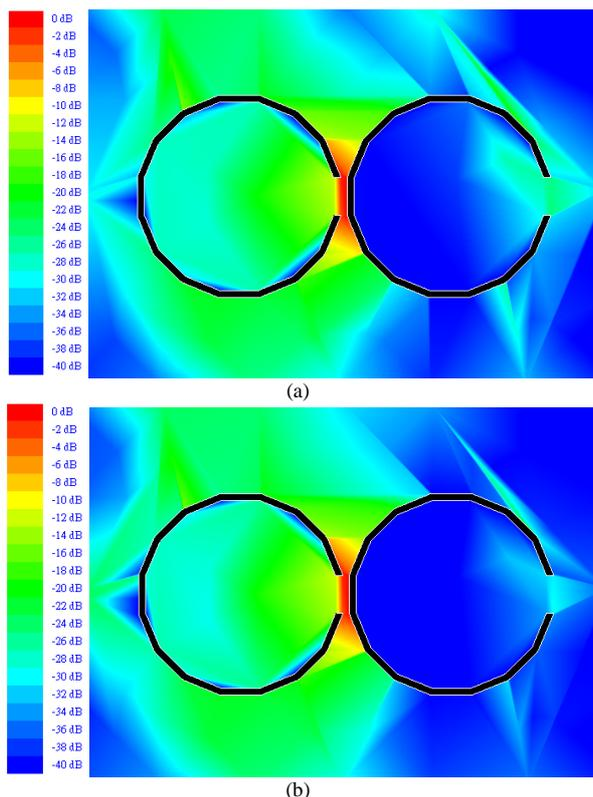
Fig. 5. Current distribution of the two slotted ground structures on the ground plane at (a) 3.75 GHz and (b) 4.32 GHz.
