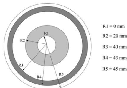
Figure 2. The configuration of cable in simulation studies
