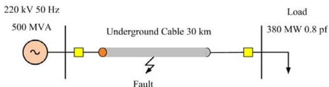
Figure 1. The system used in simulation studies
