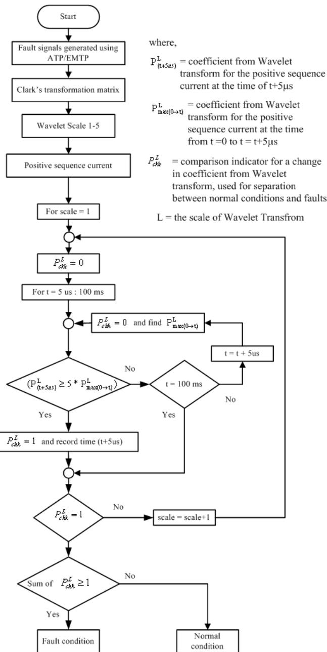
Figure 4. Flowchart for fault detection.
