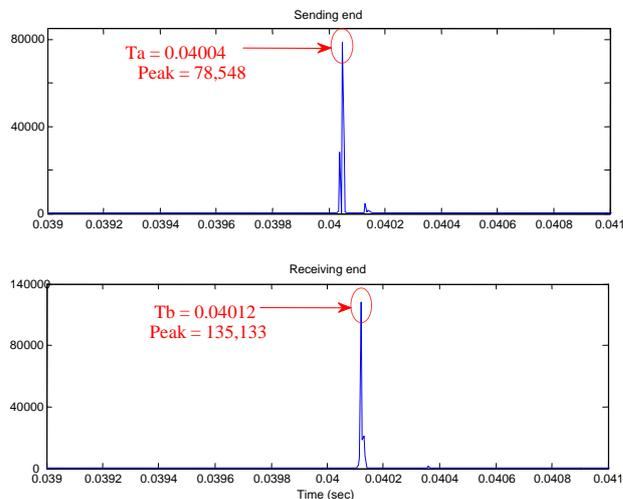
Figure 7 First peaks in the scale 1 at both ends of underground cable for the positive sequence of current signal shown in Figure 5.
