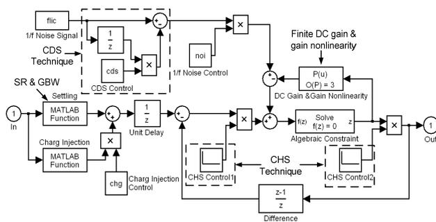
Fig.3. An improved integrator behavioral model.
