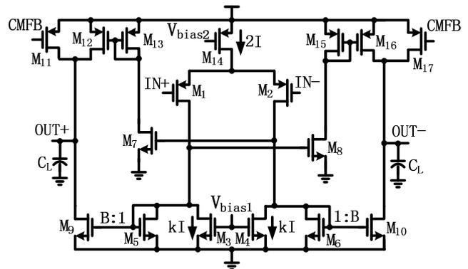
Fig.5. Schematic of the proposed class-AB current mirror OTA with the current starving technique.
