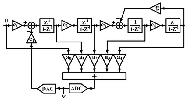
Fig.1. Single-loop 4th-order modulator topology.
