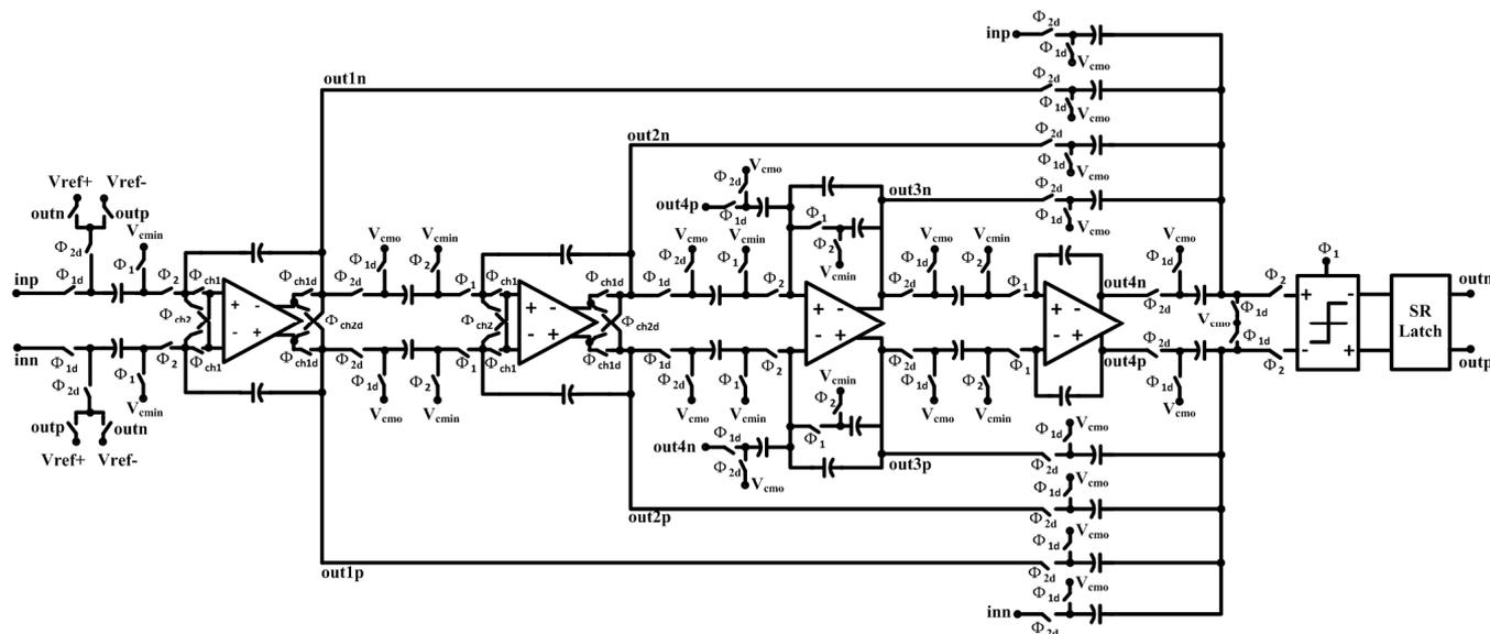
Fig. 9. Schematic of the complete proposed modulator circuit.
