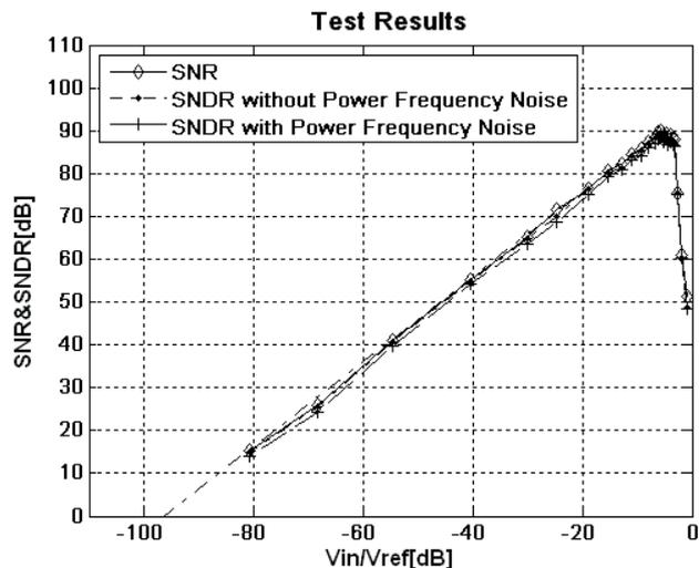
Fig.12. Measured SNR and SNDR versus input amplitude.
