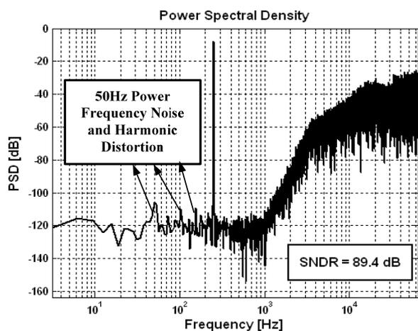
Fig.11. Measured output spectrum of the designed modulator with 40960 samples.
