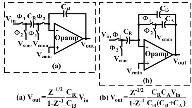
Fig.8. Schematic diagrams and transfer functions of two resonators: (a) traditional type (b) proposed type.
