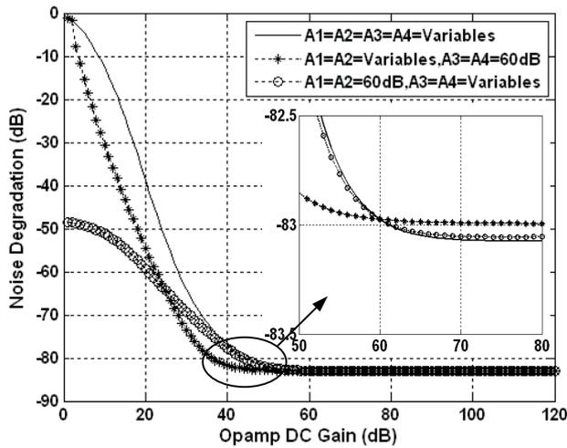
Fig. 2. Noise degradation versus different DC gain values.
