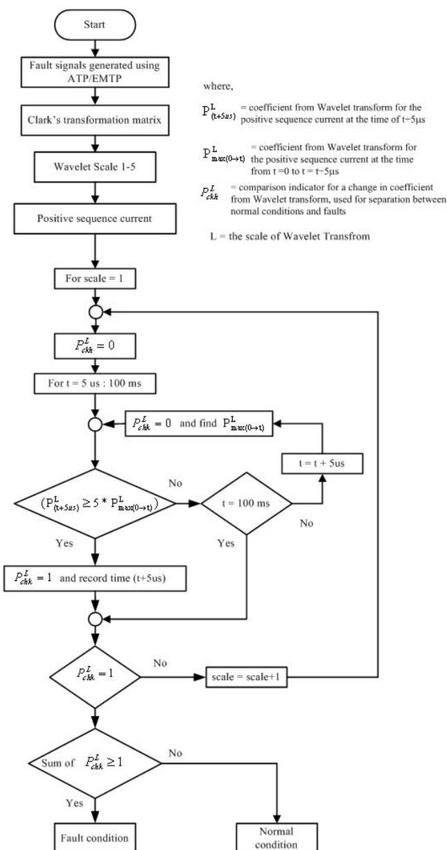
Figure 4. Flowchart for fault detection.
