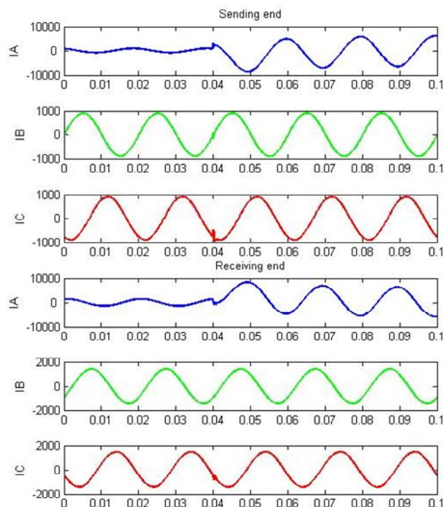
Figure 3. Example of ATP/EMTP simulated fault signals for AG fault at sending end.
