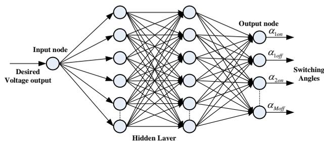
Fig. 4 ANN for optimal switching angles approximation
