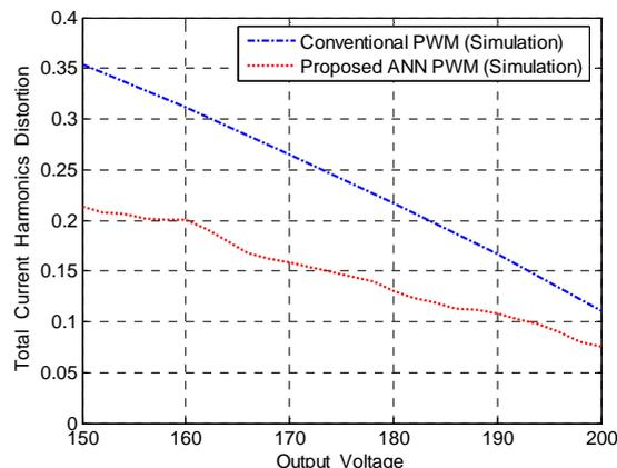
Fig.8 Comparison of  $THD_i$  from the proposed techniques, conventional technique PWM for some given desired output voltage.
