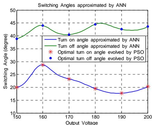
Fig.7 Optimal switching angle versus desired output voltage: Marker ‘\*’ and ‘•’ is the optimal angles evolved by PSO that use for training set, Solid line is the Approximated angles by ANN.
