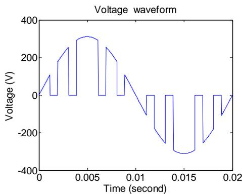
Fig.2 Output waveform of conventional fixed-duration PWM AC voltage controller. The rms voltage of this waveform is 180 V.
