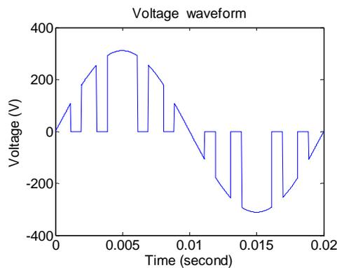
Fig.2 Output waveform of conventional fixed-duration PWM AC voltage controller. The rms voltage of this waveform is 180 V.
