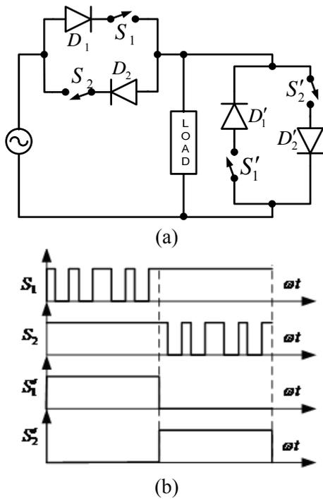
Fig.1 (a) Single-phase PWM AC voltage controller
