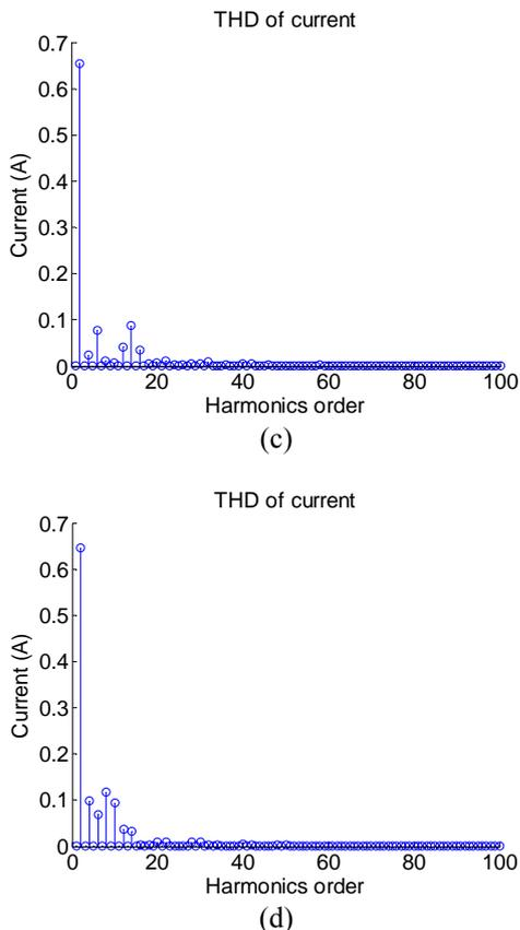
Fig.6 Output voltage waveform and current spectrum of PWM AC voltage controller for given desired voltage = 160V. Output voltage waveform of (a) PSO proposed technique, (b) conventional technique. Current spectrum of (c) PSO proposed technique, (d) conventional technique.
