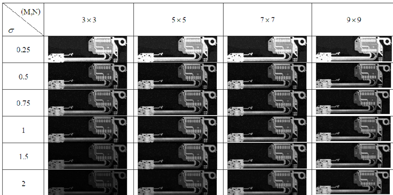
Fig. 8. Images of PCB after reducing noise with different values of \sigma , M and N
