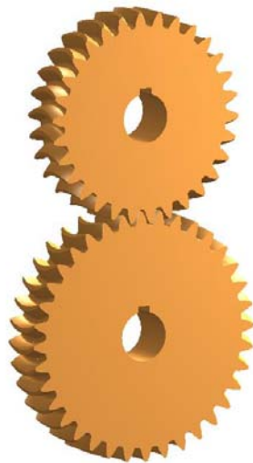
Fig.5 The solid model of the modified curvilinear gear set
