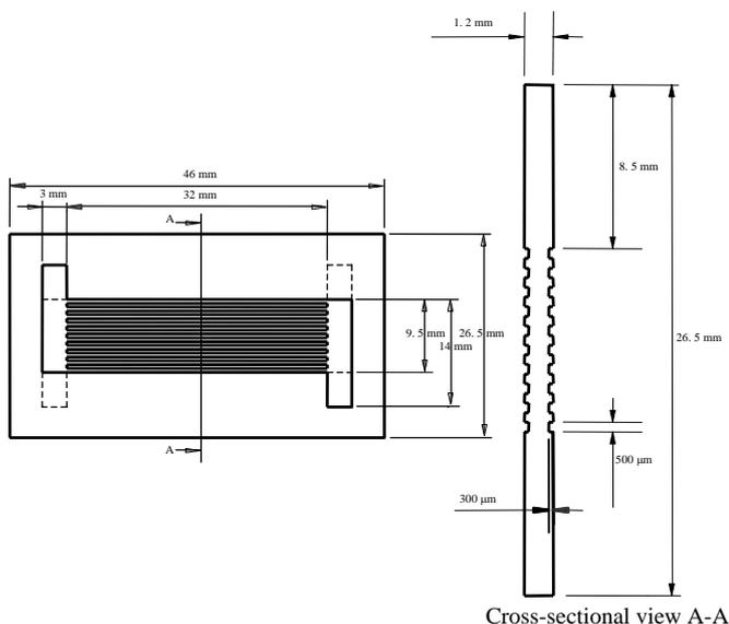
Fig. 2. Dimensions of the test section
