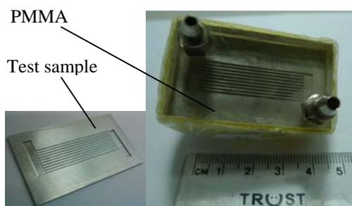
Fig. 3. A photo of the microchannel heat exchanger
