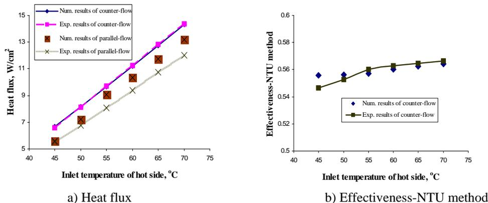
Fig. 7 A comparison between numerical and experimental results
