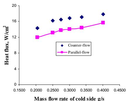
Fig. 9. A relationship between the heat flux and the mass flow rates of the cold side
