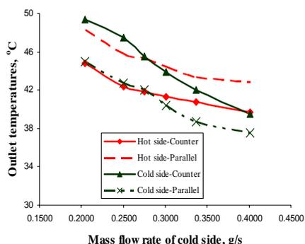
Fig. 8. A relationship between the outlet temperatures and the mass flow rates of the cold side
