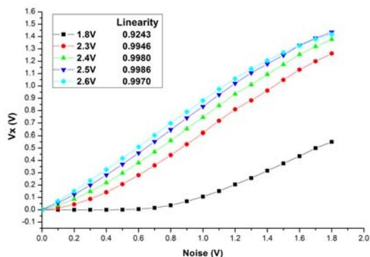
Fig. 4 Analysis of various charging supply voltage for higher PSN detection linearity
