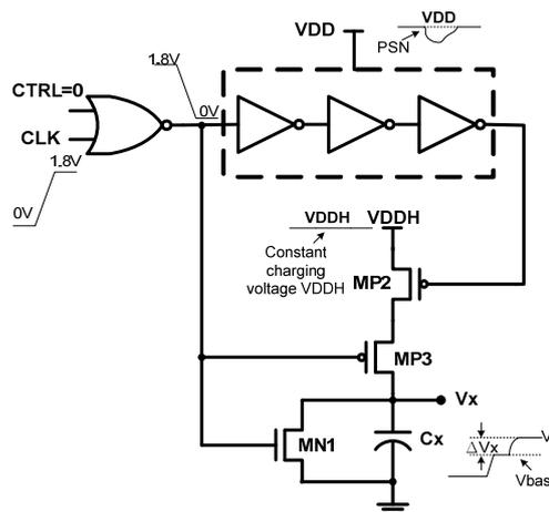
Fig. 2 The proposed power supply noise detection circuit
