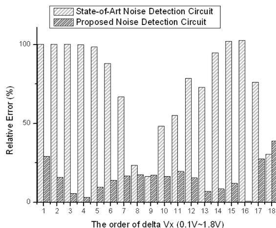
Fig. 6 Comparison of PSN detection error in the state-of-art PSN detector in [6] and the proposed PSN detector
