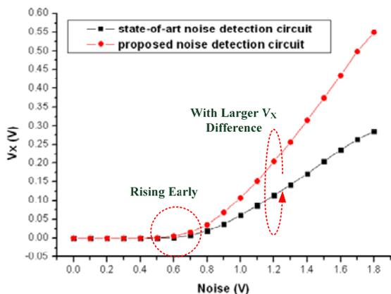
Fig. 3 Comparison of  $V_x$  variation under various power supply noise pulse amplitude in the proposed PSN detection circuit versus the state-of-art PSN detector in [6]
