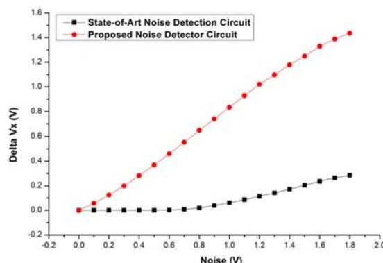
Fig. 5 Comparison of detected output voltage difference in the state-of-art PSN detector in [6] and the proposed PSN detector
