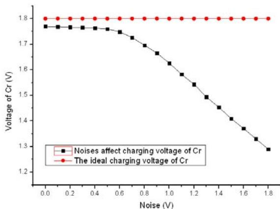
Fig. 1 The analysis of charging voltage variation of  $C_r$  along with various PSN amplitudes
