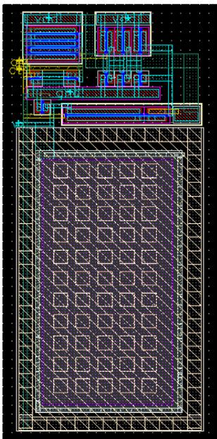
Fig. 7 Chip layout of the proposed PSN detector
