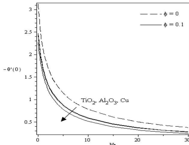
Fig. 1. Variations of  $-\theta'(0)$  with  $Nr$  for different types of nanoparticles when  $Pr = 6.2, m = 0$  and different  $\phi$ .
