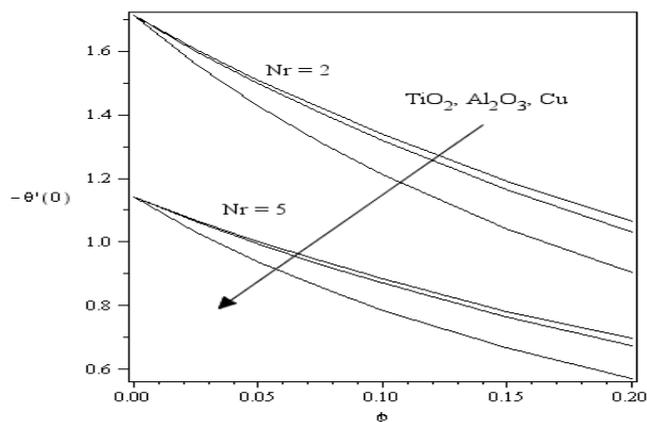
Fig. 2. Variations of  $-\theta'(0)$  with  $\phi$  for different types of nanoparticles when  $Pr = 6.2, m = 0$  and different  $Nr$ .
