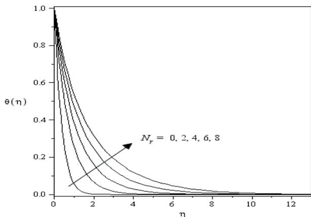
Fig. 4. Temperature profiles for  $\text{Al}_2\text{O}_3$  nanoparticles with  $m = 0$ ,  $\phi = 0.1$  for various  $Nr$ .
