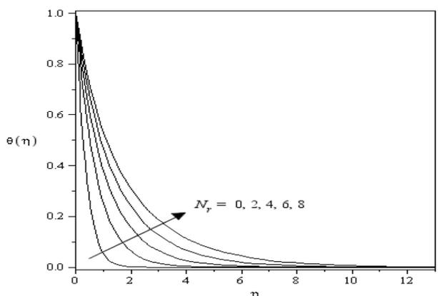
Fig. 5. Temperature profiles for  $\text{TiO}_2$  nanoparticles with  $m = 0$ ,  $\phi = 0.1$  for various  $Nr$ .
