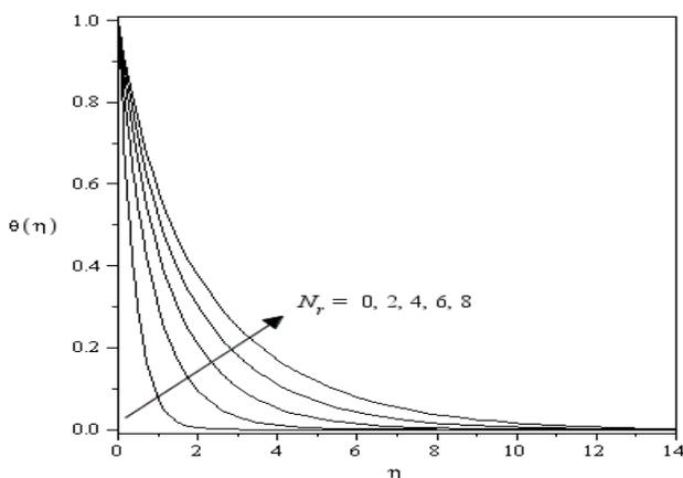
Fig. 3. Temperature profiles for Cu nanoparticles with  $m = 0, \phi = 0.1$  for various  $Nr$ .
