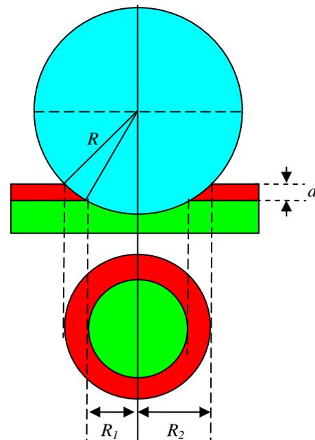
Fig 1. Schematic illustration of ball crater method for coating thickness measurements.
