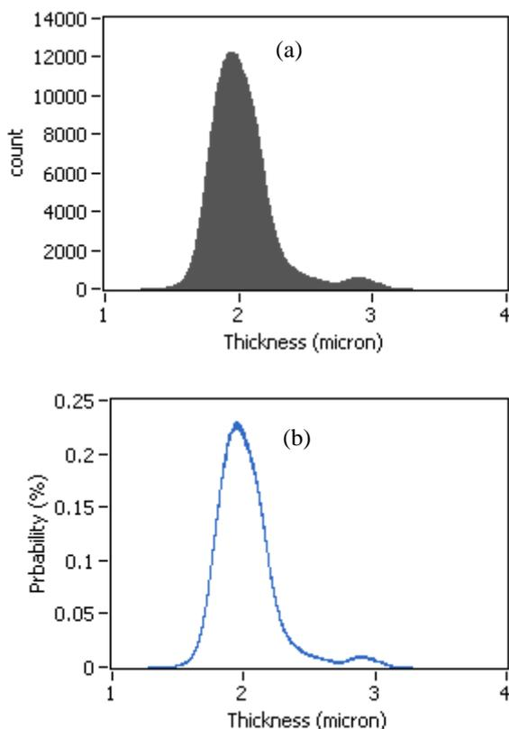
Fig. 5. (a) Histogram and (b) probability distribution of thickness values obtained by a traditional method (estimated by using the 5319006 combinations of all points from the top and bottom circular boundaries in Fig. 4).
