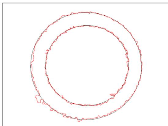
Fig. 4 Best fit circles on the two edges of the crater.
