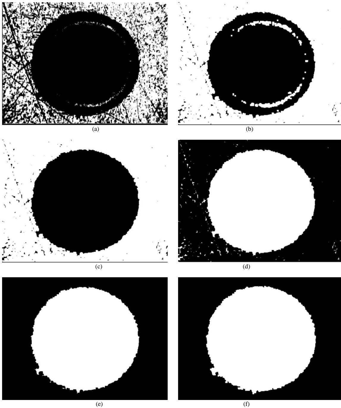
Fig. 3. Intermediate stage images when processing Fig. 2(a) to obtain Fig. 2(b): (a) thresholding; (b) dilation; (c) low pass filtering; (d) image inversion; (e) low pass filtering; (f) dilation.
