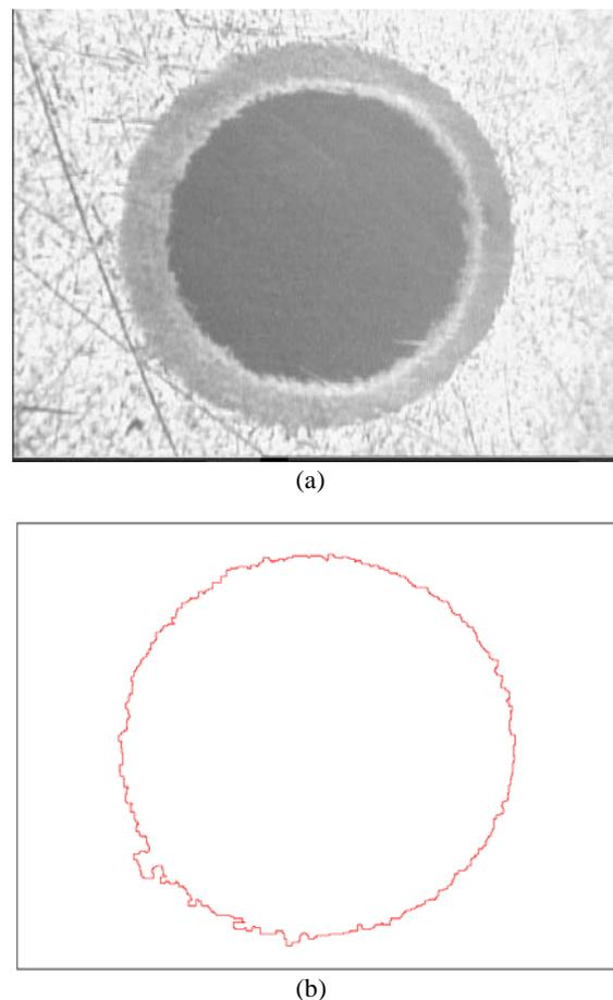
Fig. 2. (a) Crater image and (b) top circle edge of a coating sample (a titanium alloy substrate, a pure, metallic interlayer and a multi-element alloy topcoat) viewed under a microscope with  $\times 10$  objective magnification.
