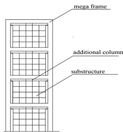
Fig.2 Mega-sub controlled structure system
