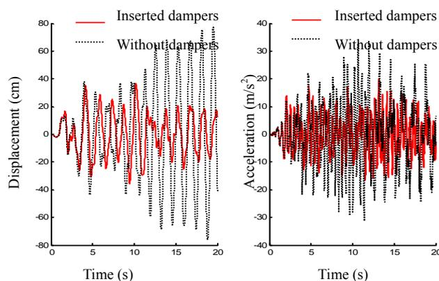
Fig.10 Displacement and acceleration time history curve of the top floor in the main structure
