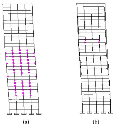
Fig.8 Distribution of plastic hinges under rare earthquake (e.g. peak acceleration value is 400gal)
