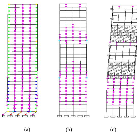
Fig.9 Distribution of plastic hinges under super rare earthquake (e.g. peak acceleration value is 1000gal)
