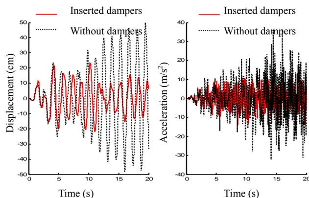
Fig.11 Displacement and acceleration time history curve of first substructure
