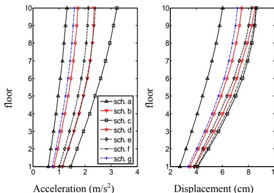
Fig.6 storey acceleration and displacement envelope diagram in the first substructure
