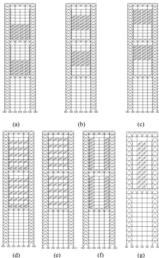
Fig.5 seven arranging schemes of friction dampers
