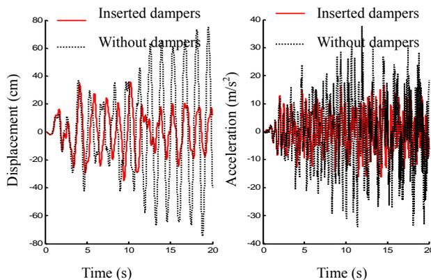
Fig.12 Displacement and acceleration time history curve of second substructure
