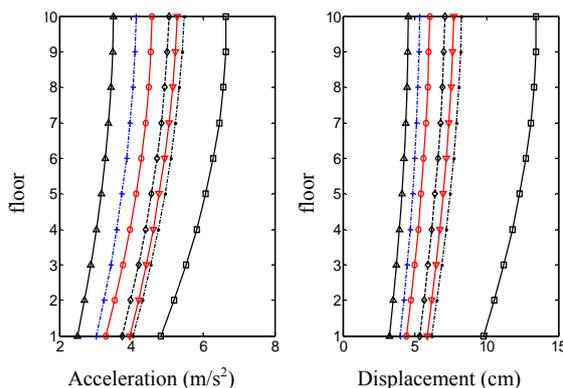
Fig.7 storey acceleration and displacement in the second substructure
