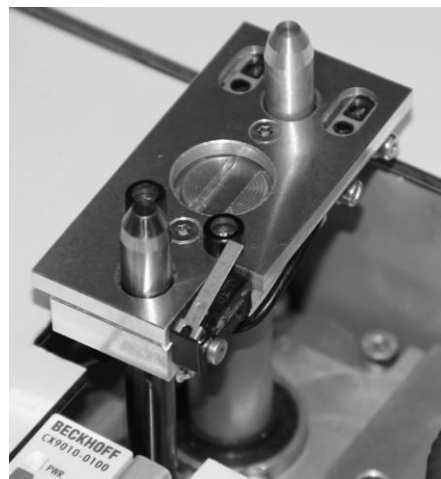
Fig. 3. Connector for towing trolleys
