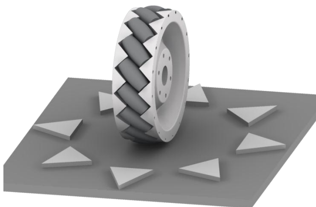
Fig. 2. Omnidirectional Mecanum wheel
