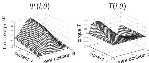
Fig. 2. Magnetic flux and torque functions of current and rotor position
