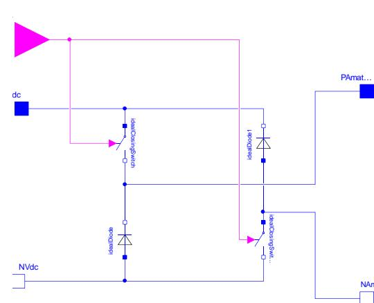
Fig. 9. Asymmetric bridge power converter
