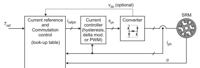
Fig. 7. Schematic current based torque control
