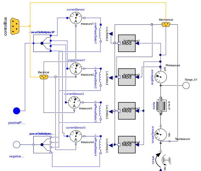
Fig. 5. Rotor model from a 12 rotor poles switched reluctance machine
