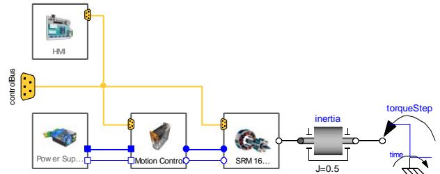
Fig. 13. Testrig of a 16/12 switched reluctance machine
