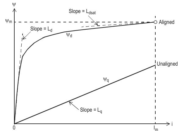
Fig. 3. Aligned and unaligned magnetization curves for building SRM analytical model
