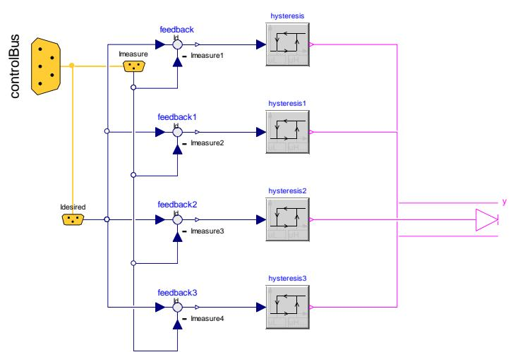
Fig. 10. Implementation of current controller
