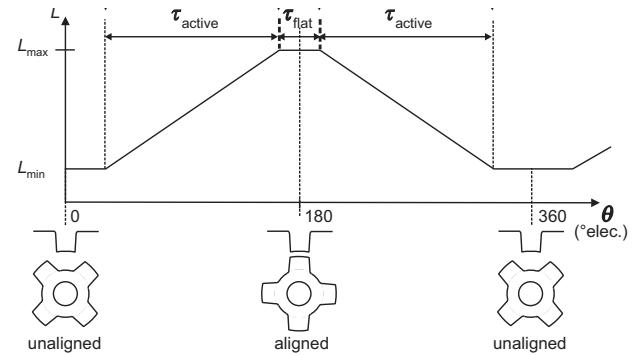
Fig. 1. Ideal inductance function of rotor position
