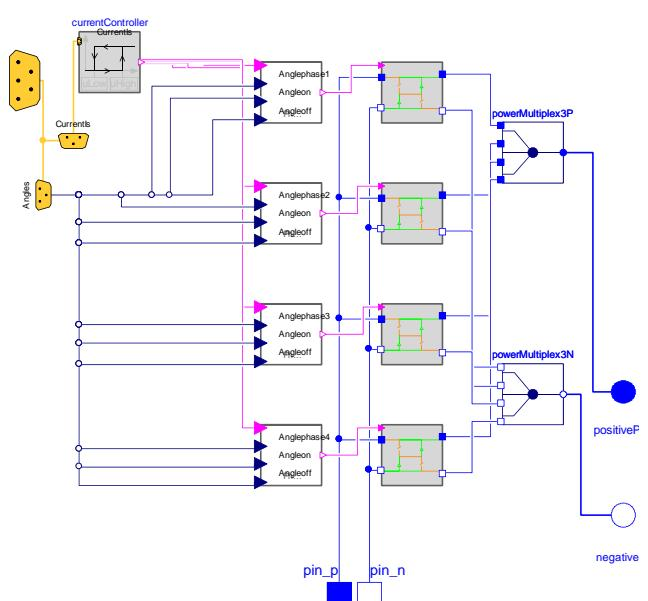
Fig. 11. Control unit for a 4 phase switched reluctance machine
