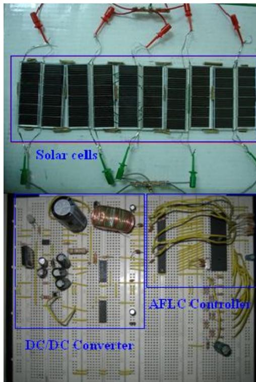
Fig.15 Hardware of PV System for MPPT
