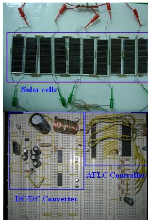
Fig.15 Hardware of PV System for MPPT
