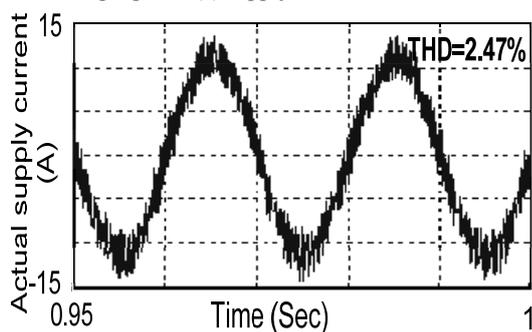
Fig.10 phase (a) supply current for the proposed method
