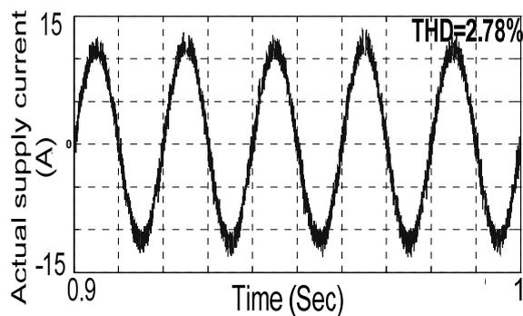
Fig.12 phase (a) supply current for SDM
