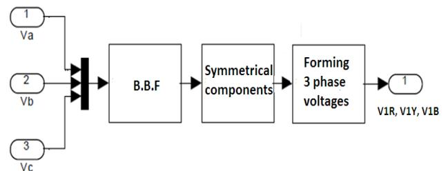
Fig.2 Block diagram of the positive sequence detector.
