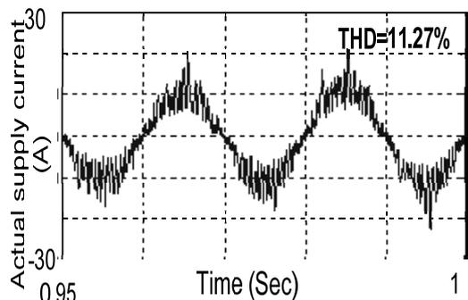
Fig.9 phase (a) supply current for IRPT
