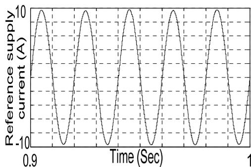
Fig.7 phase (a) reference current for SRF
