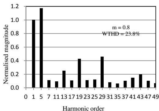
Fig. 17. Harmonic spectrum for Line Voltage (before elimination)
