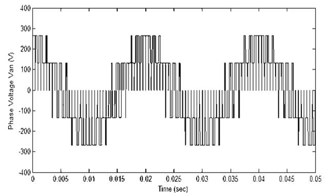
Fig. 13. Line to neutral Voltage ( $m = 0.8$ )
