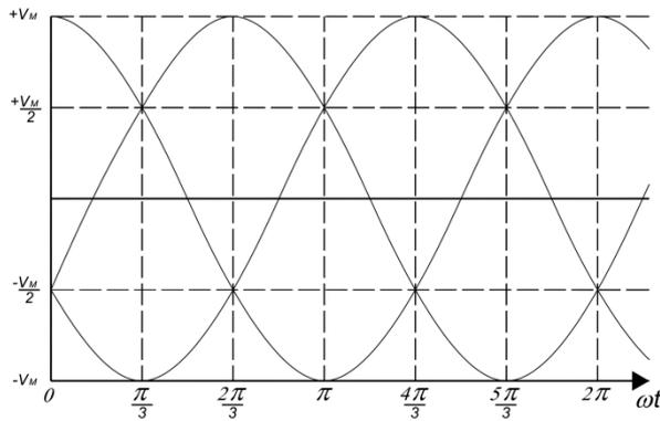
Fig.5 Inverter phasor angular positions in fundamental cycle
