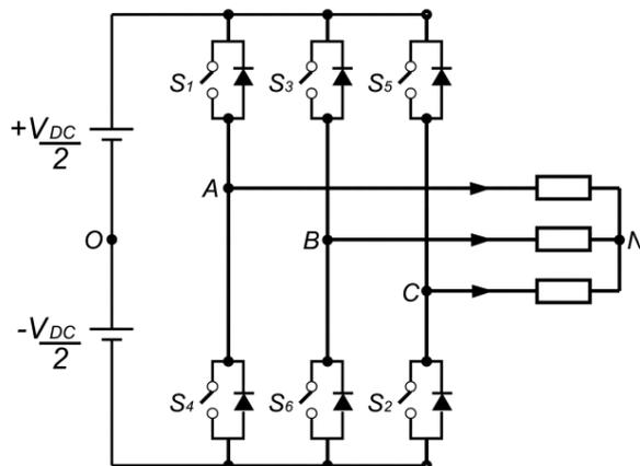
Fig. 2. Three phase voltage source inverter configuration
