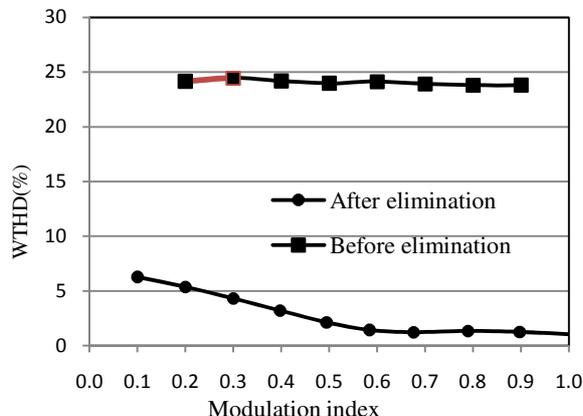
Fig. 20. Line voltage WTHD Vs Modulation index
