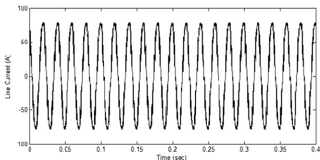
Fig. 16. Line current for m = 0.8
