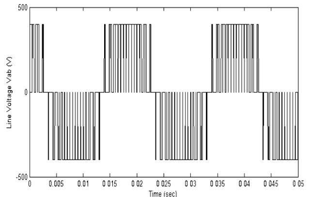
Fig. 14. Line to line Voltage ( $m = 0.8$ )
