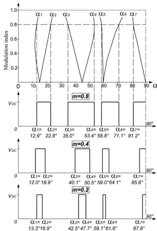
Fig. 18. Selective Harmonic Elimination (m = 0.8, 0.4 & 0.2)
