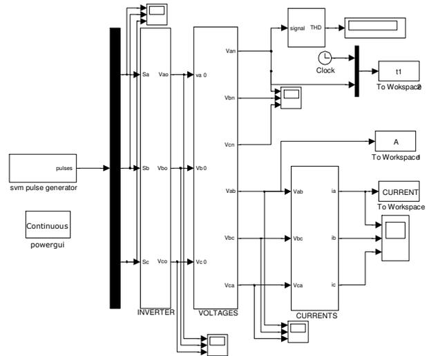
Fig. 11. MATLAB/Simulink model of three phase inverter based on SVM
