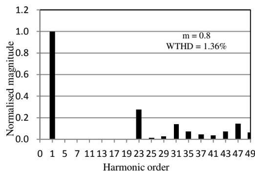
Fig. 19. Harmonic spectrum for Line Voltage (after elimination)
