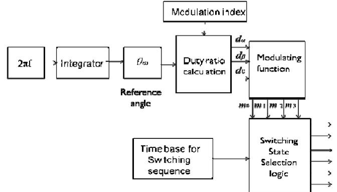
Fig. 7. Block diagram for SVM pulse generation
