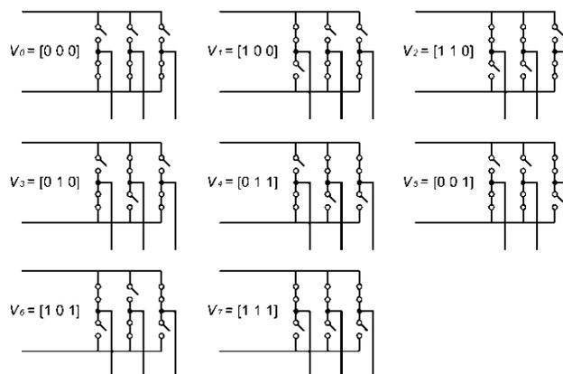
Fig. 3. Inverter switching topology
