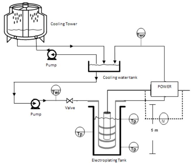
Fig. 2 A cooling system for a hard chrome plating process.
