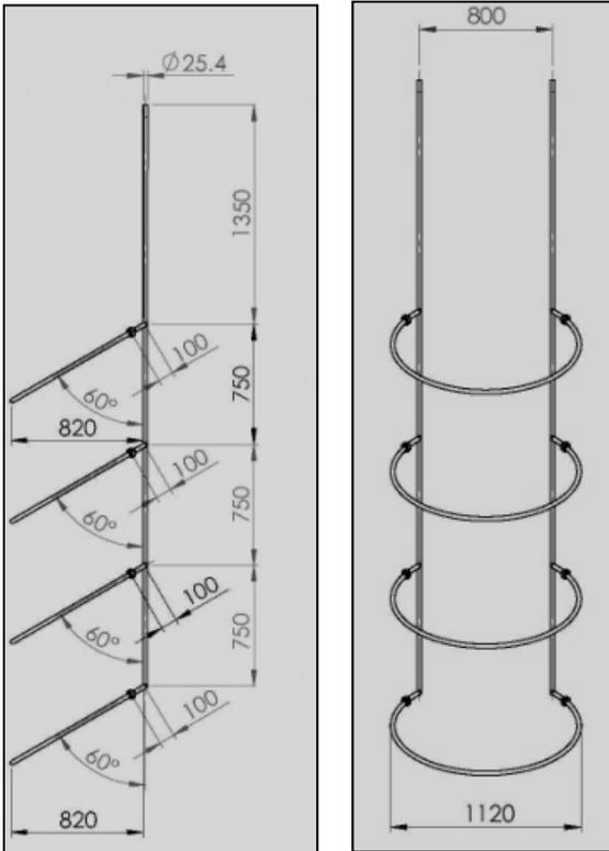
Fig. 1 The front/side view of the new design structure
