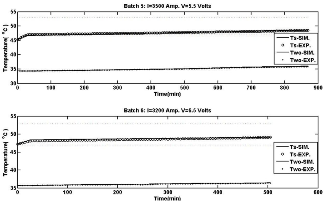
**Fig. 4** The temperature profile of the plating solution and the water out with actual plant data of a vibration type coiled-tube heat exchanger batch 5 and 6.
