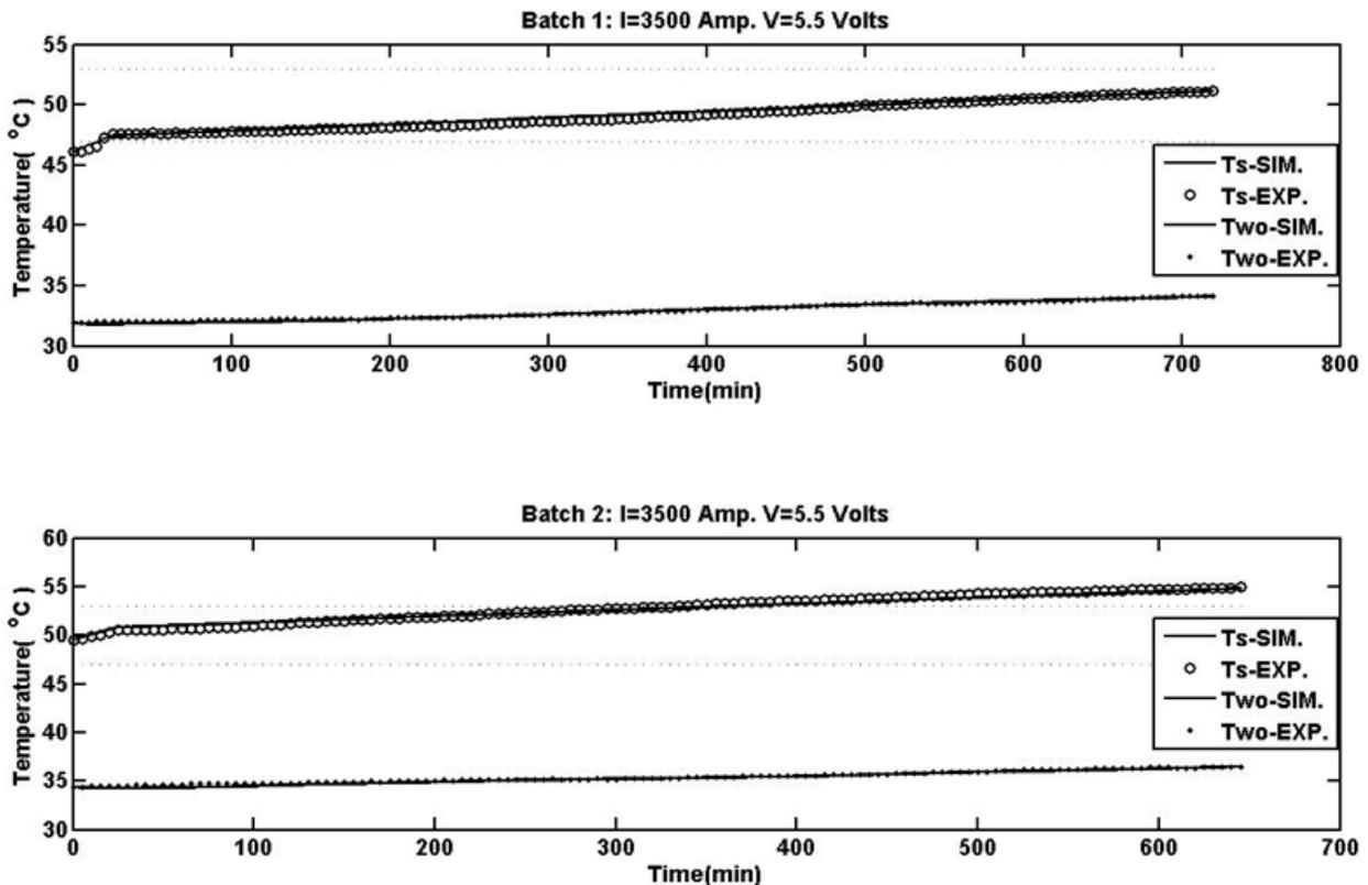
Fig. 3 The temperature profile of the plating solution and the water out with actual plant data of the U-tube heat exchanger batch 1 and 2.
