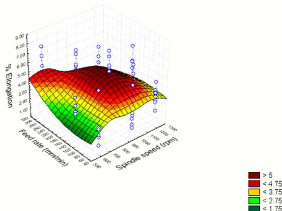
Fig 9: Surface plot relating percentage elongation, spindle speed and feed rate for all the welds.
