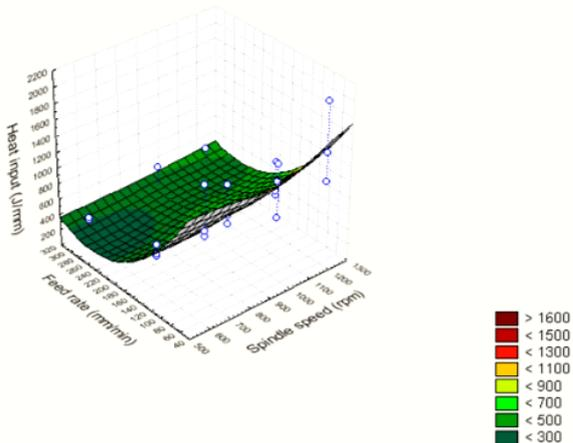
Fig 7: Surface plot relating heat input, spindle speed and feed rate for all the welds.
