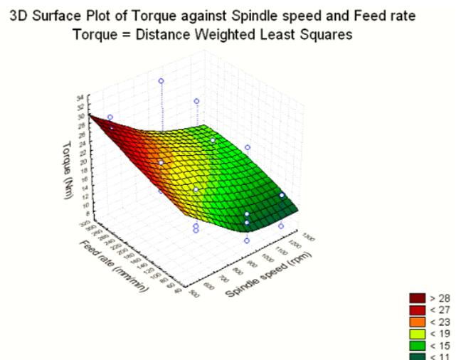
Fig 6: Surface plot relating torque (T), spindle speed and feed rate for all the welds.
