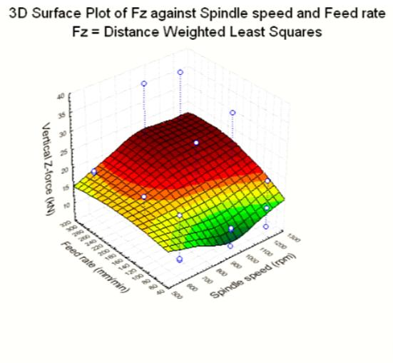
Fig 5: Surface plot relating vertical force (Fz), spindle speed and feed rate for all the welds.
