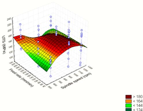
Fig 8: surface plot relating UTS, spindle speed and feed rate for all the welds
