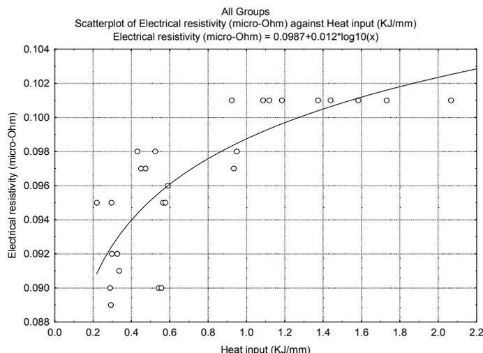
Fig 2: Scatter plot of electrical resistivity versus heat input for all the welds produced.
