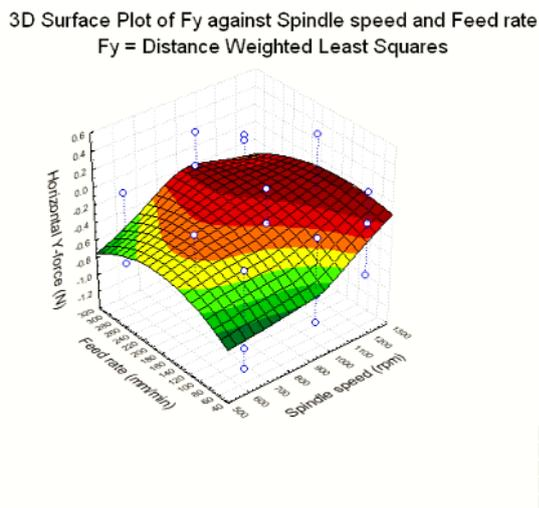
Fig 4: Surface plot relating horizontal force Fy, spindle speed and feed rate for all the welds.
