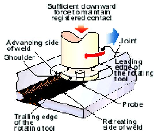
Fig. 1: Schematic diagram of friction stir welding process [3]
