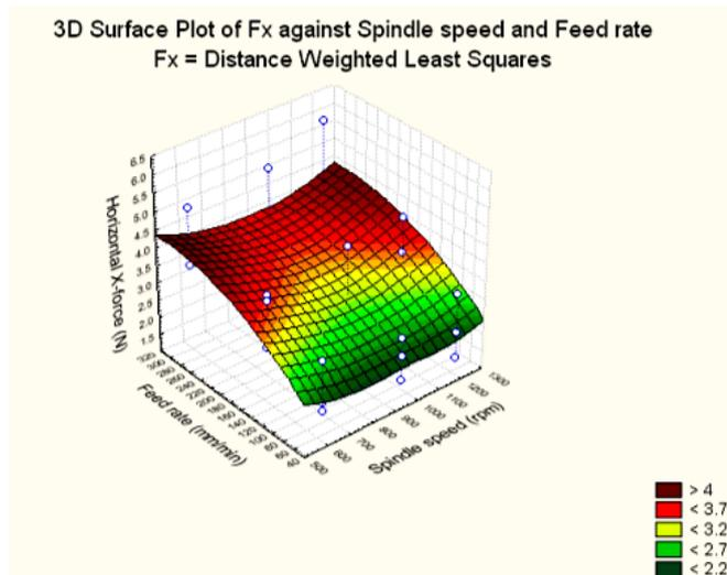
Fig 3: Surface plot relating horizontal force (Fx), spindle speed and feed rate for all the welds.
