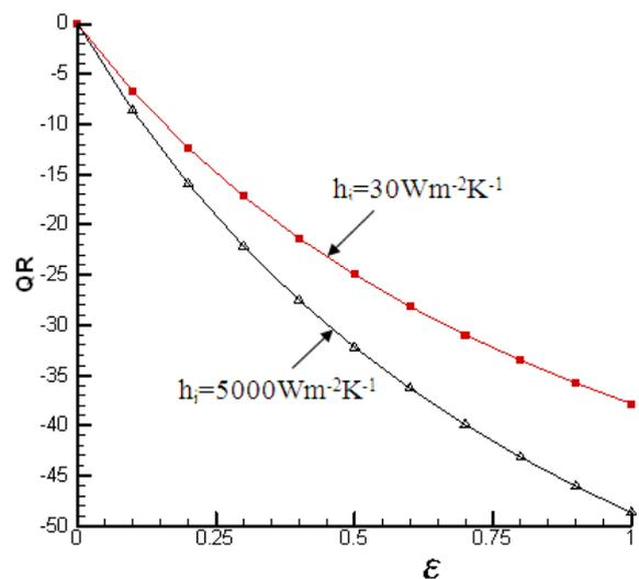
Fig. 4 The relations between heat transfer rate error, QR, and emissivity,  $\varepsilon$ , for a heater
