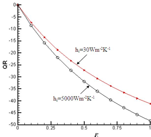
Fig. 6 The relations between heat transfer rate error,  $QR$ , and emissivity,  $\epsilon$ , for a chiller
