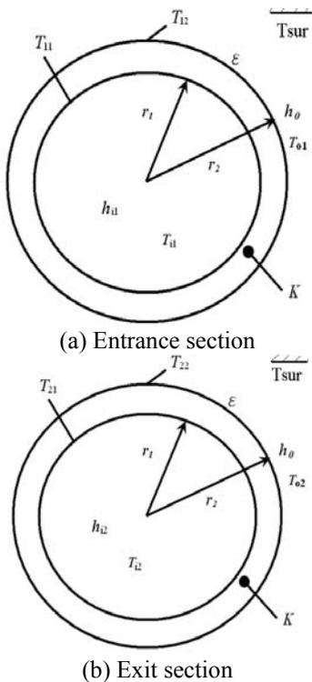
Fig. 3 A single-pipe heat exchanger and its relative parameters at entrance and exit sections
