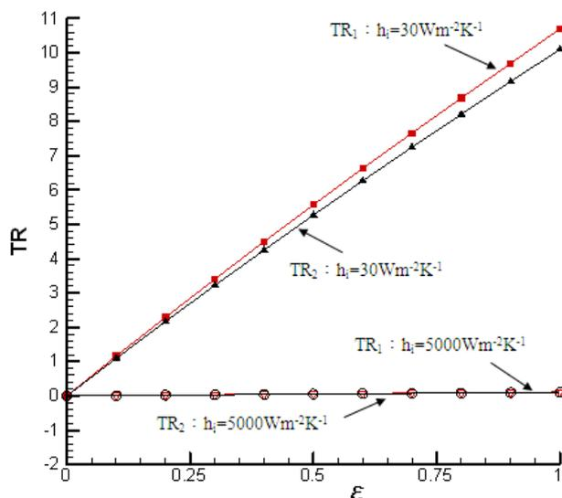
Fig. 5 The relations among surface temperature errors,  $TR_1$  and  $TR_2$ , and emissivity,  $\epsilon$ , for a heater
