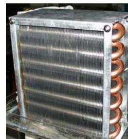
**Fig. 1** Condenser or evaporator of air conditioner is a single-pipe heat exchanger
