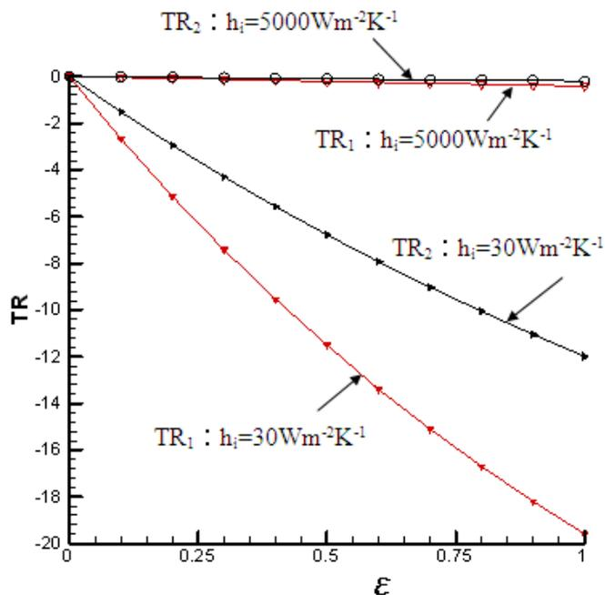
Fig. 7 The relations among surface temperature errors,  $TR_1$  as well as  $TR_2$ , and emissivity,  $\epsilon$ , for a chiller
