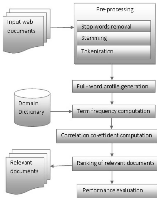
Fig. 1 Architectural design of the proposed work
