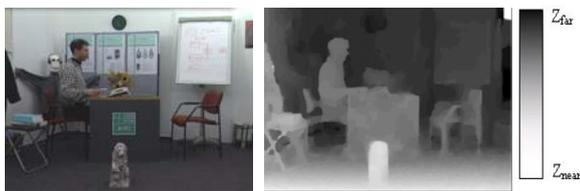
Fig. 2. Video-plus-depth representation; left: texture image, right: depth image.
