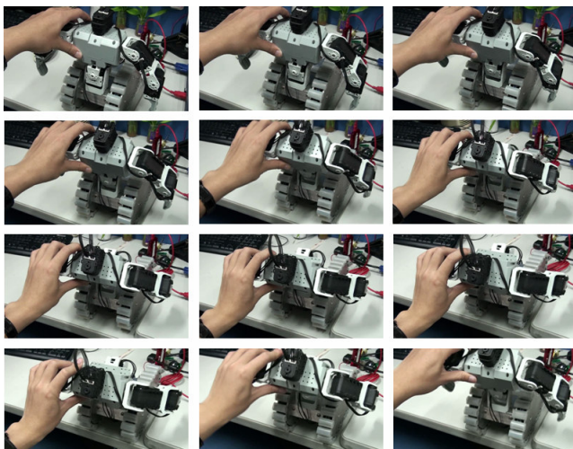
Fig. 10. Compliant behaviors of the mobile robot.
