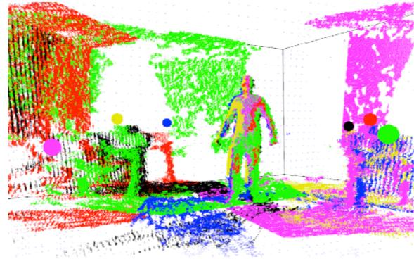
Figure 4: Result from the global calibration. Point clouds from six cameras are merged in a global coordinate system. The cameras (shown in circle) and their corresponding point clouds are color-coded.
