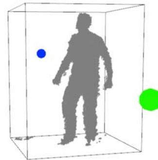
Figure 5: Result from the background subtraction. The estimated bounding box used to segment the model is shown along with the complete 3D model. It can be seen that the segmentation works really well in separating the foreground from the background.
