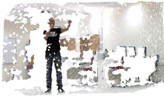
Figure 3: A dynamic 3D point cloud from one camera with the depth to color mapping.
