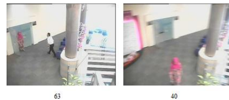
Fig. 7. Sample of sharp and blurred images (left and right). Number below each image is the average edge magnitude for the image. The magnitude is higher in sharp image.
