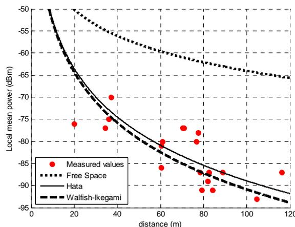
Fig.3. Measured vs. Predicted values
