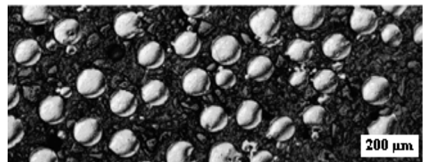
Figure 3: Morphology of Ti6Al4V powder
