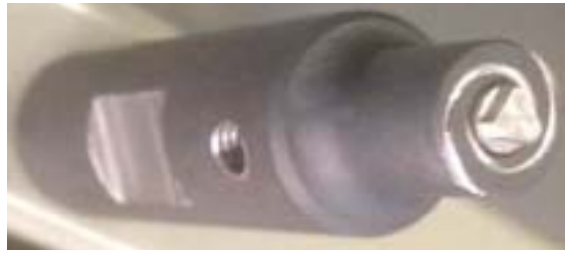
Figure 1. Scroll shoulder Triflat (TFT) FSW tool having pin with three equidistant flats (tool).
