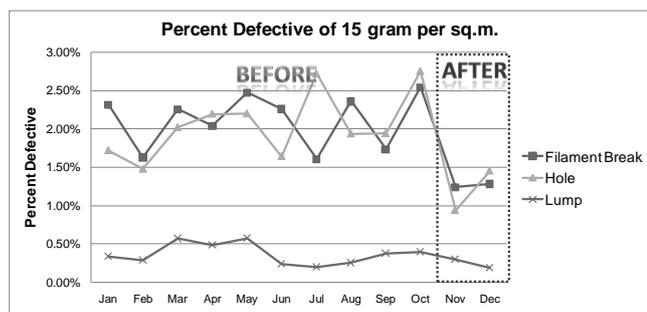
Fig.11. The percent defective of 15-gsm fabric before and after improvement.
