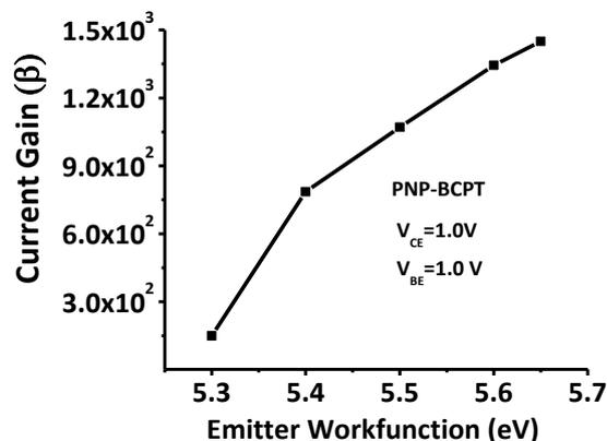
Figure 8: Variation of current gain with Emitter work-function
