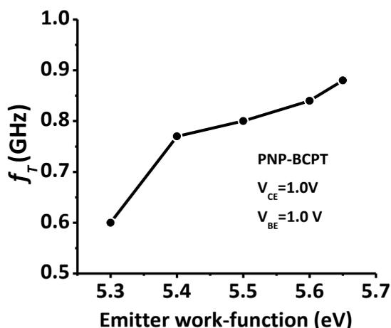
Figure 9: Variation of cutoff frequency ( $f_T$ ) with Emitter work-function
