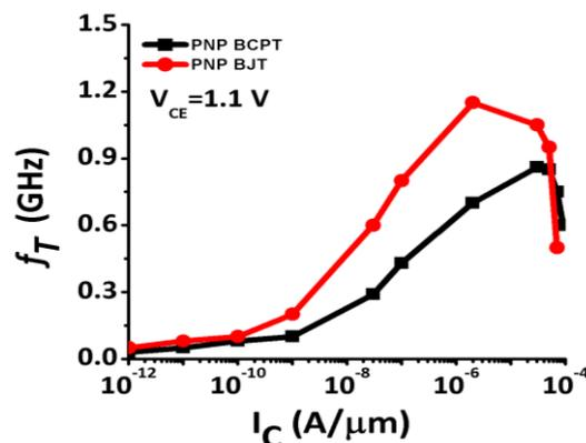
Figure 6: Cutoff frequency ( $f_T$ ) comparison of the conventional *pnp* BJT, *pnp* BCPT structures.
