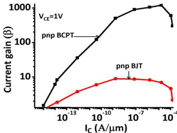
Figure 5: Current gain comparison of the conventional *pnp* BJT, *pnp* BCPT structures.
