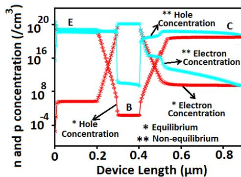
Figure 2: Total carrier concentration in the proposed *pnp* BCPT structure for different bias conditions (under thermal equilibrium and under non-equilibrium conditions).
