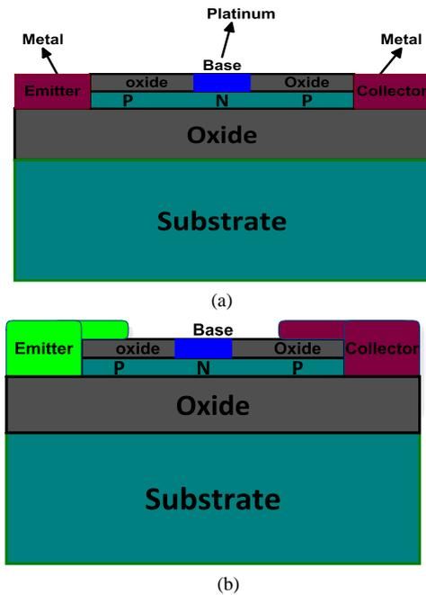
Figure 1: Schematic diagrams of (a) Conventional BJT and (b) Proposed *pnp* BCPT.
