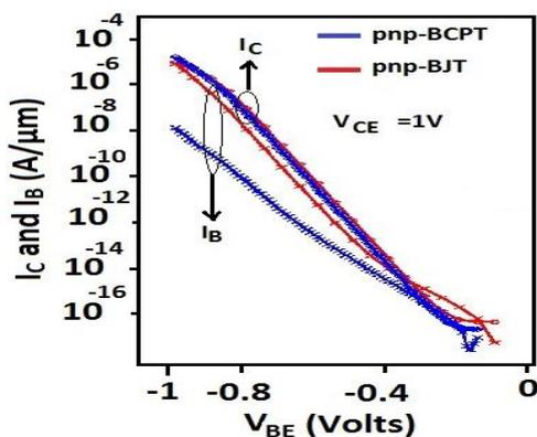
Figure 4: Gummel plots for the conventional *pnp* BJT and the proposed *pnp* BCPT structures.
