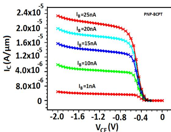
Figure 7: Output Characteristics of proposed *pnp* BCPT
