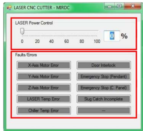
Fig. 6. GUI for the LASER power controller.
