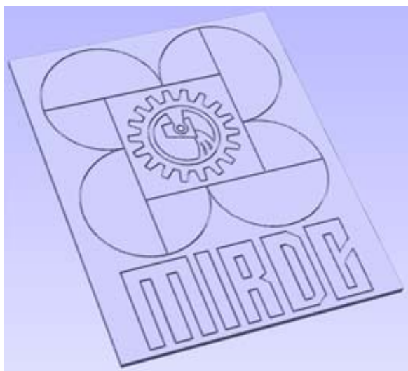
Fig. 18. Toolpath produced in VCarve Pro in .plt.
