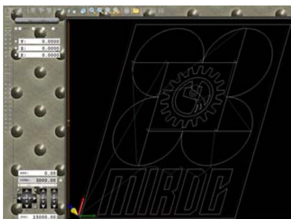
Fig. 19. Toolpath produced in CNC USB Controller.
