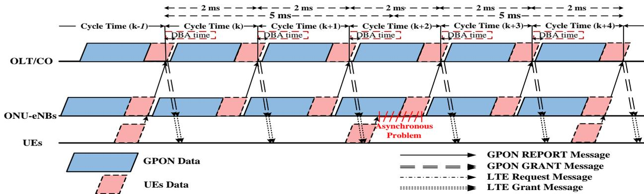
Figure 2(a). Asynchrony Problems in Integrated GPON-LTE Network.
