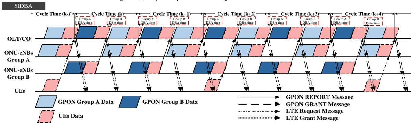
Figure 2(b). Synchronous Interleaved Dynamic Bandwidth Assignment.
