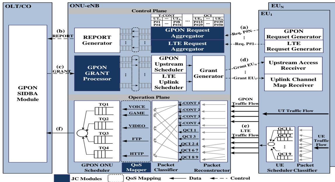
Figure 1. Interoperations of Function Modules for GLCNA.
