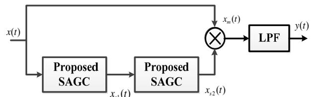
Fig. 2. Large carrier AM demodulation block diagram based SAGC scheme
