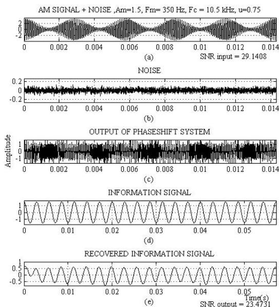
Fig. 6. The result of AM demodulation system using the proposed sinusoidal automatic gain control scheme based the Hilbert transform for white noise environment where (a), (b), and (c) are the AM signal, noise and the output of the proposed AGC scheme, respectively, (d) and (e) are the information signals at the transmitter and receiver, respectively.
