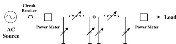
(b) The  $\pi$ -equivalent model used for experimental setup.
