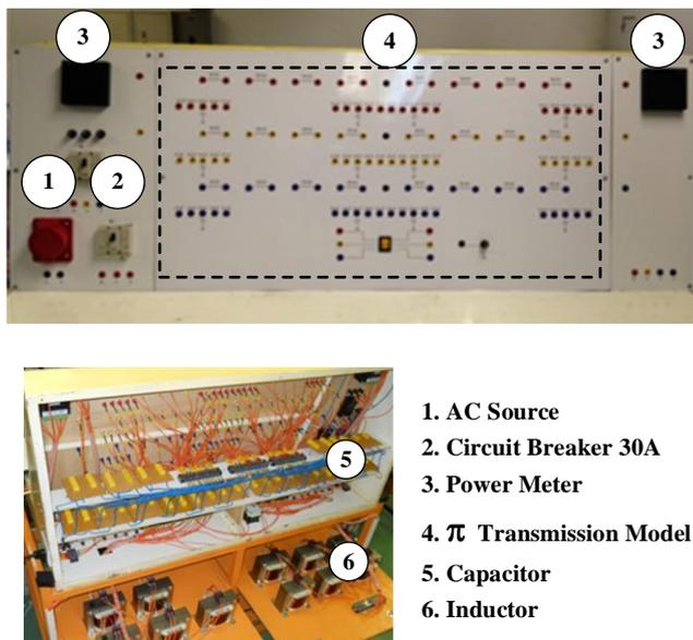
Fig.2. The panel of experimental setup.
