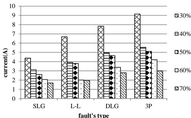
Fig.9. Results of fault current for various fault types and various fault locations from the experimental setup in case of load of 60W.
